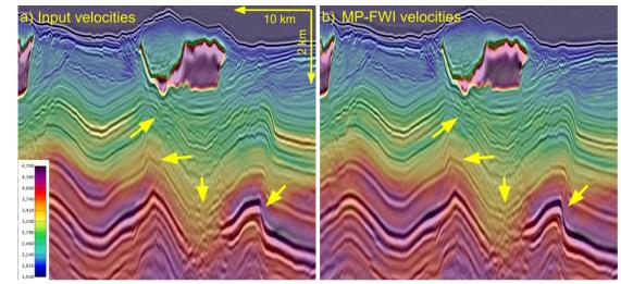
Figure 2: Input MP-FWI imaging velocity model co-rendered with a Q-RTM of pre-processed data (a) and output MP-FWI imaging velocity model co-rendered with a corresponding Q-RTM of pre-processed data (b).
