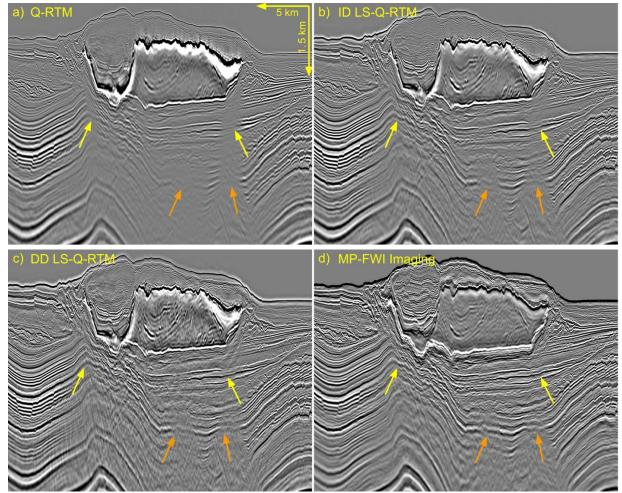
Figure 3: Mirror Q-RTM (a), image-domain LS-Q-RTM (b) and data-domain LS-Q-RTM (c) of the pre-processed down-going wavefield and MP-FWI imaging derived reflectivity (d).
